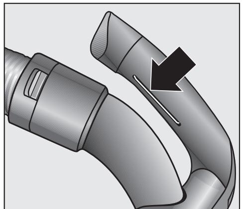
**!** When vacuuming, in particular fine dust, e.g. sawdust, sand, plaster, flour, talcum powder etc., electrostatic charges build up naturally. Under certain conditions these charges will be released. To avoid the unpleasant effects of these discharges, a metal inlay has been incorporated into the underside of the handle. Please make sure that you keep your hand in constant contact with this metal strip during vacuuming.
