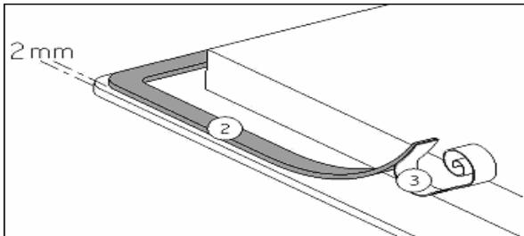
Stick the gasket (2) two millimeters from the external edge of the glass, after removing the protection sheet (3).
